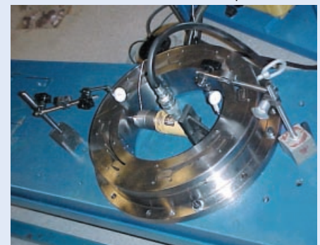
Experimental Setup To Measure Damper Stiffness
