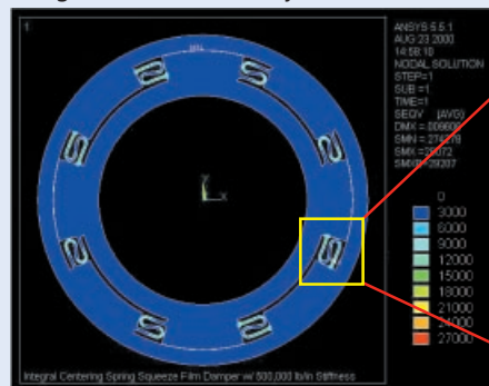
Integral Centering Spring Squeeze Film Damper with 500,000 lb./in. Stiffness Designed Using Finite Element Analysis
